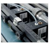
Rotary tools Up to four perforating heads are available: all of them plug and play. The setup will be done within just a few seconds on the touchscreen control panel.
