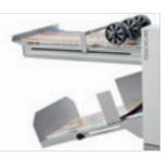
of two different output levels. For creasing and folding, the upper delivery belt is used. For creasing only the lower reception
