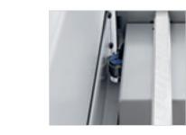
Double sheet detection A professional ultrasonic double sheet detection system which offers a 100% control of all sheets running through the machine.
