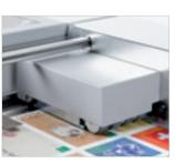
Vacuum pile feeder The pile feeder is using a vacuum belt technology and air knife control for a perfect sheet separation. It handles paper sizes from 105 x 148 mm to 375 x 1'050 mm.
